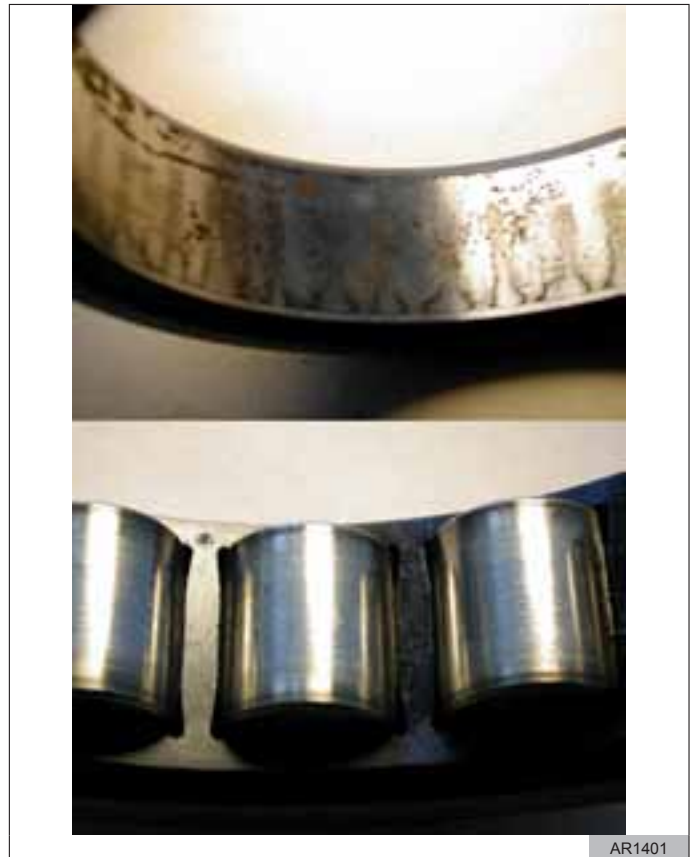
Figure 29 Overheated roller bearing elements
