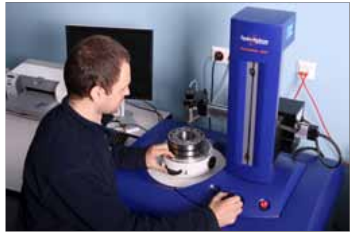
Figure 16 Measurements carried out on a Talyrd 365 device
