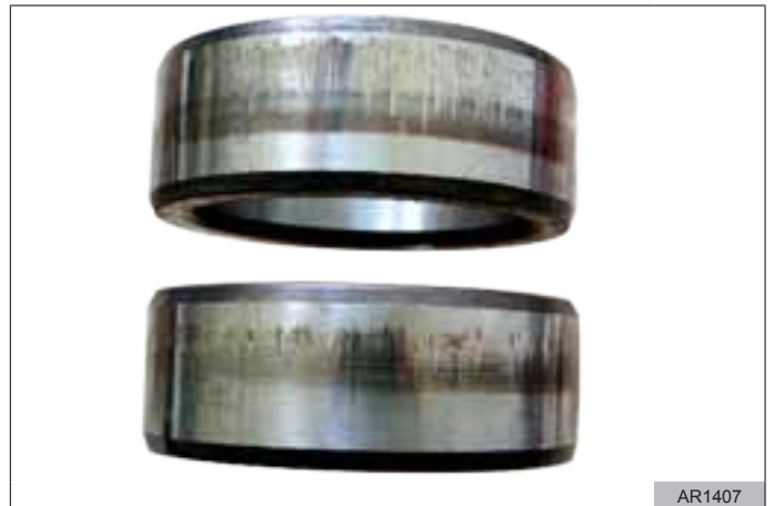
Figure 35 Pits on the raceways of bearings' inner rings
