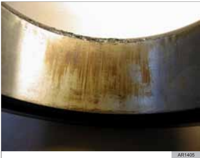
Figure 33 Tears in the outer race of bearing due to corrosion
