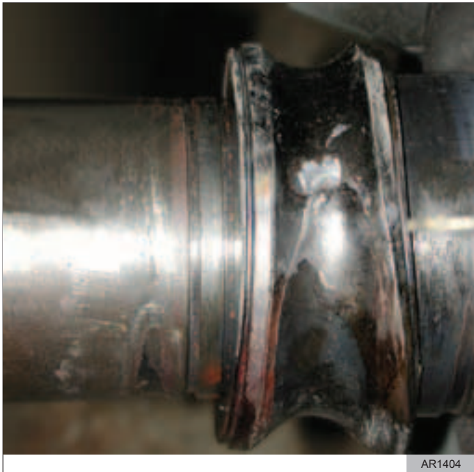
Figure 32 Overheating of a bearing as a result of too tight a fit in its housing
