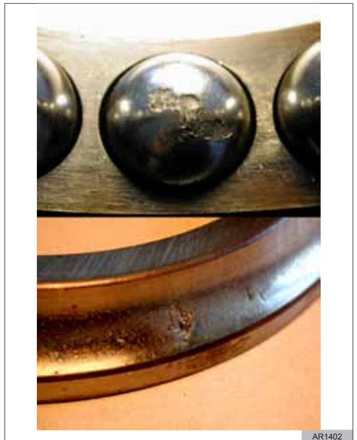
Figure 30 Visible material fatigue in a bearing element
