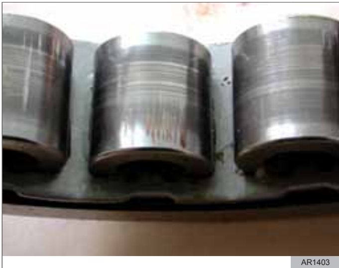
Figure 31 Indentations and scratches on rollers can arise when a roller bearing's inner ring has been obliquely pressed into the outer ring with its rollers
